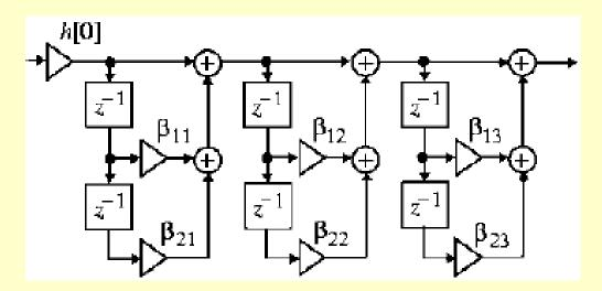
Each second-order section in the above structure can also be realized in the transposed direct form
